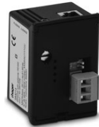
SM214: Ethernet + Gateway RS485 JBUS/MODBUS
